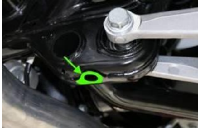
measuring point rear axle
